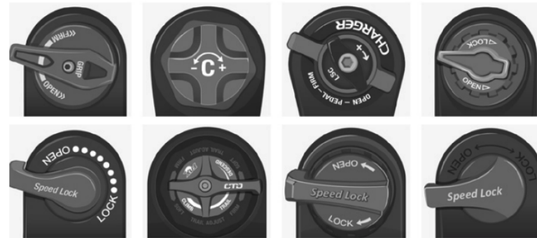
Figure 19: Different systems of fork lockouts.
