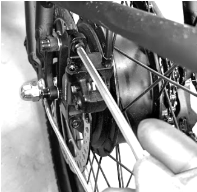
Figure 23: Undo the mount bolts to remove calliper
