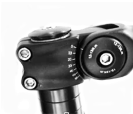
Figure 11. Loosen the M5 Bolt (center)
