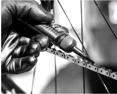
Figure 18: Applying lubricant to the chain
