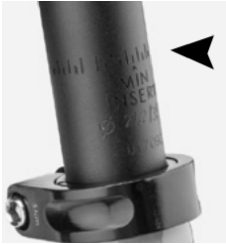
Figure 3.Min insert level seatpost
