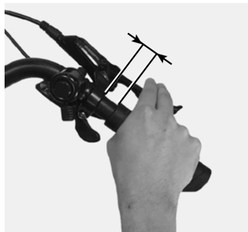
Figure 8. Distance between lever and grip
