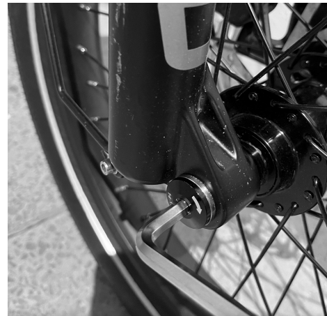
Figure 15: Tighten the axle to 15Nm
