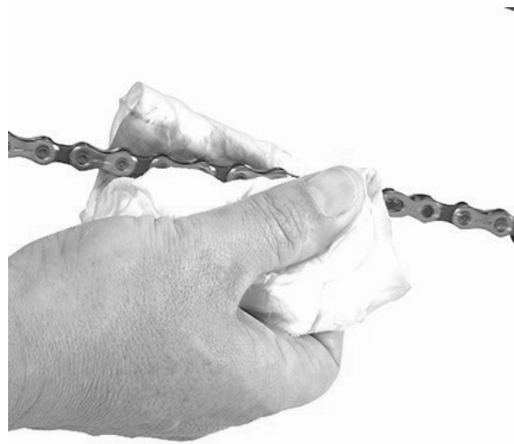
Figure 17: Use a cloth to remove debris and dirt from the chain. Gently turn the pedal with the rear wheel elevated for cleaning. Soapy water is the best cleaning solution. Avoid heavy degreasers where possible.
