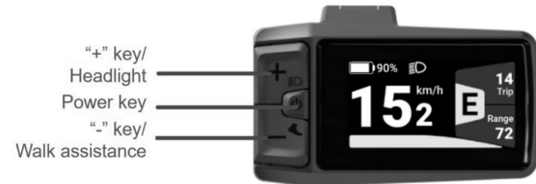
Figure 27: Press and hold button to turn on
