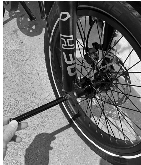
Figure 14: Installing the front wheel axle
