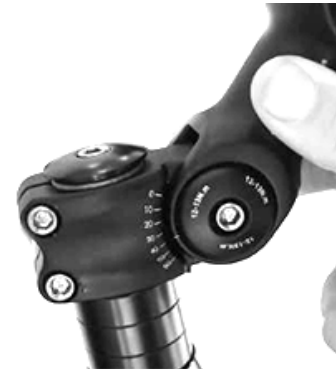
Figure 12. Adjusting the stem to position
