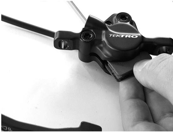
Figure 25: Gently push at the top of the pads and the pads should slide out
