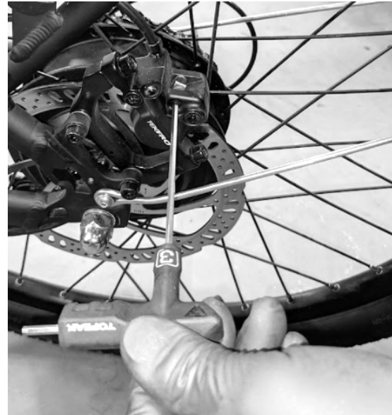
Figure 24: Undo pad retaining bolt
