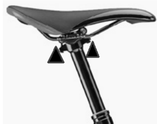
Figure 4. Intermediate saddle setback position
