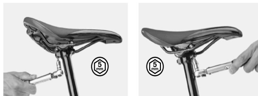
Figure 6. Tightening / loosen single saddle bolt
