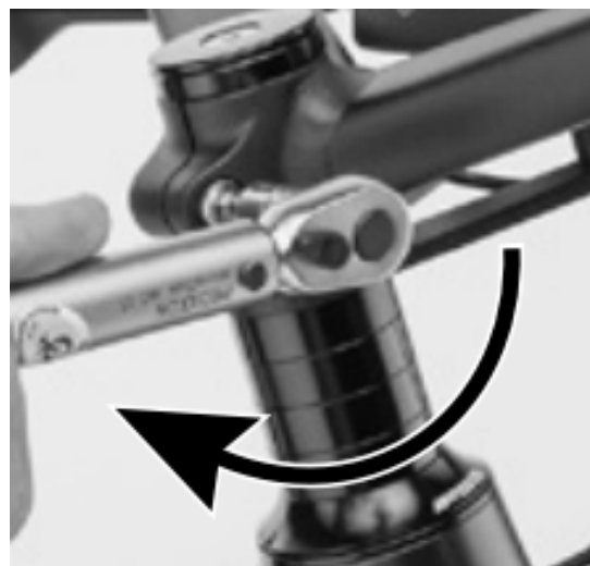
Figure 10. Retighten the stem bolts to 5nm
